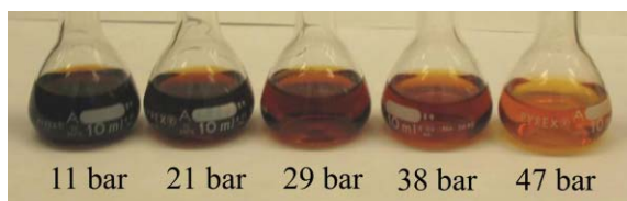
Fig. 1 Fractionation of organosolv lignin in methanol with increasing CO 2 pressures.
