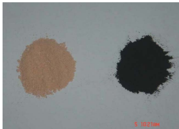
Fig. 1 Catalyst samples before (left) and after (right) argon glow discharge plasma reduction.
